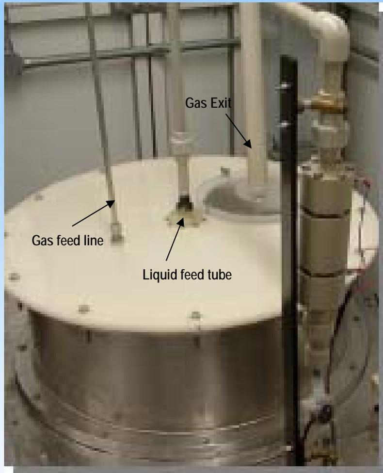
30cm SDR with built-in conductivity monitor for measuring ion depletion during conversion
