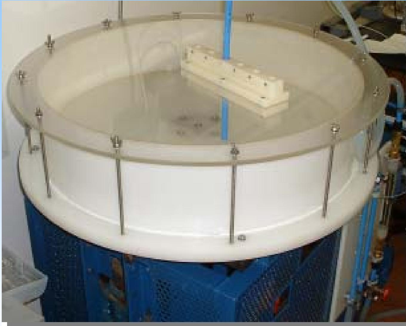
Lab Test - 30cm Disc for 10 - 40 ml/s (0.6 - 2.4 litres/min)
