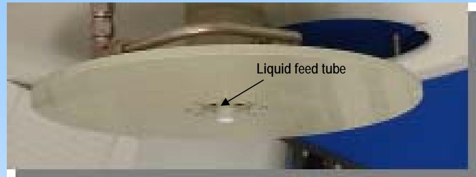
Polypropylene shroud plate to direct gas flow over the rotating disc.
