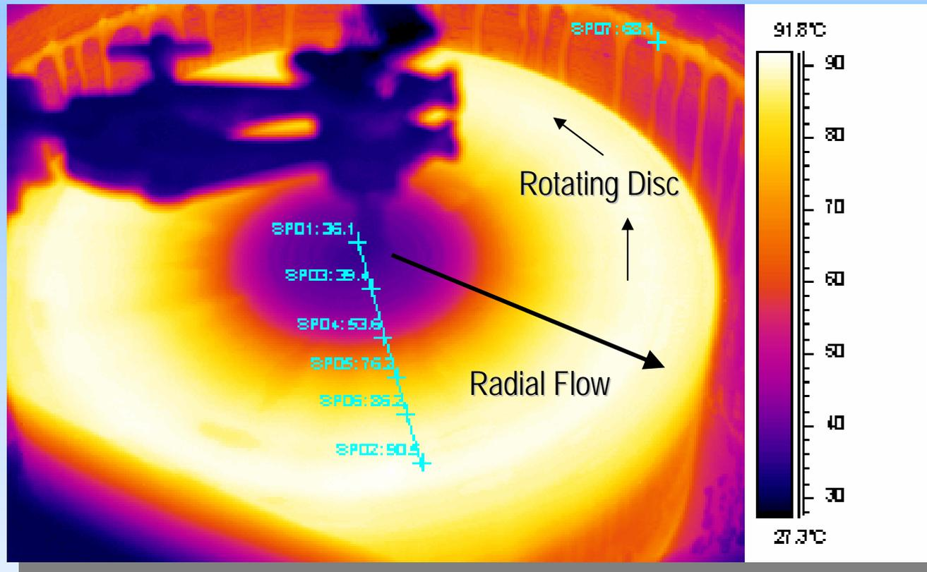
Continuous heating of "Treacle" from 40°C to 90°C in seconds using a SDR
