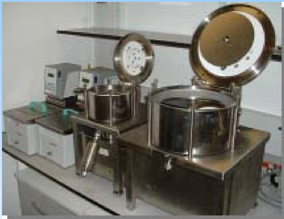
Fluid Heated / Cooled Reactors
