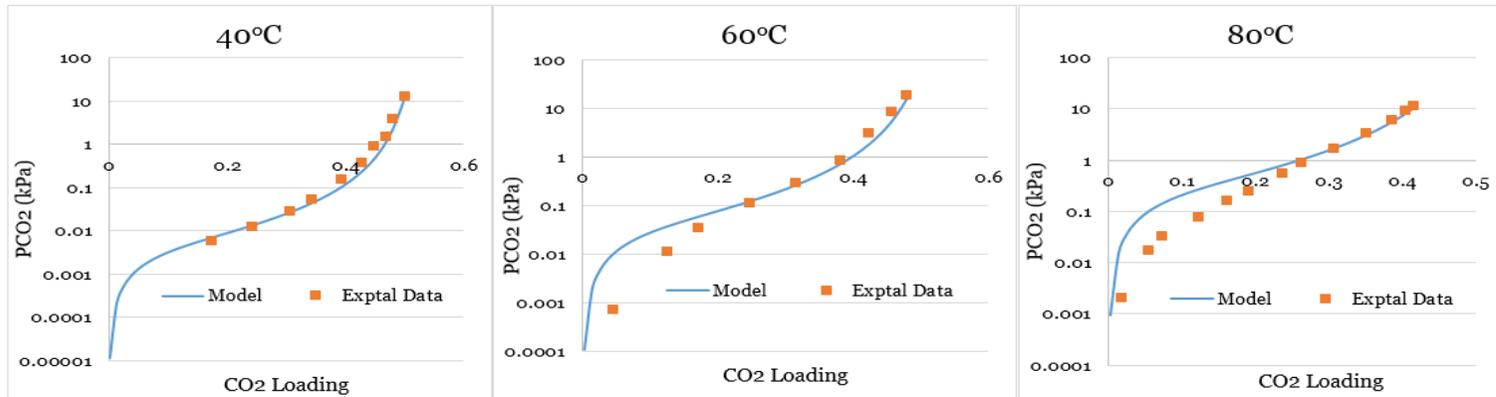
Model prediction for 60 wt% MEA solution with data from Aronu *et al.* (2011)
