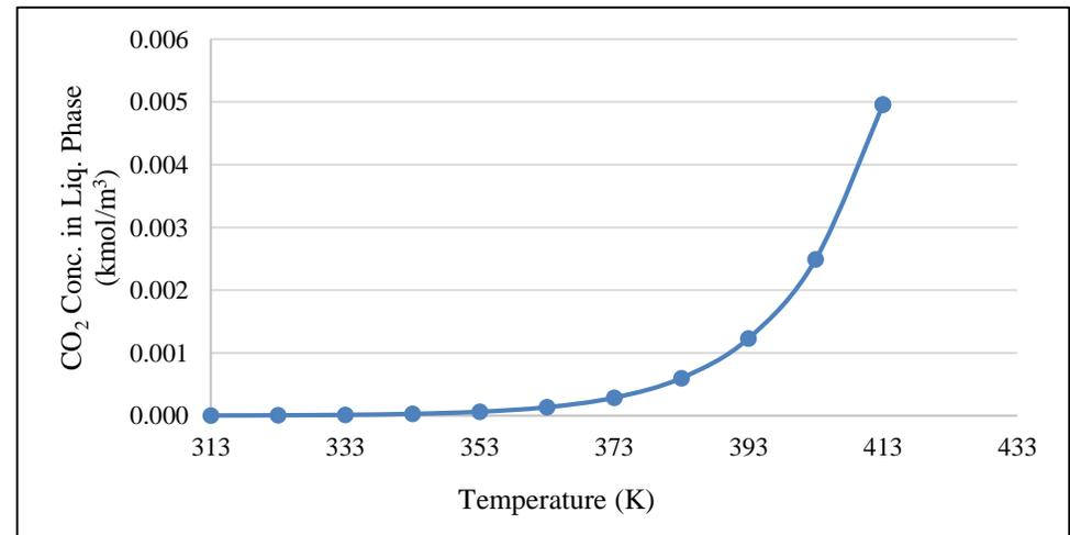
Liquid phase CO<sub>2</sub> concentration for 55 wt% MEA at an initial loading of 0.2
