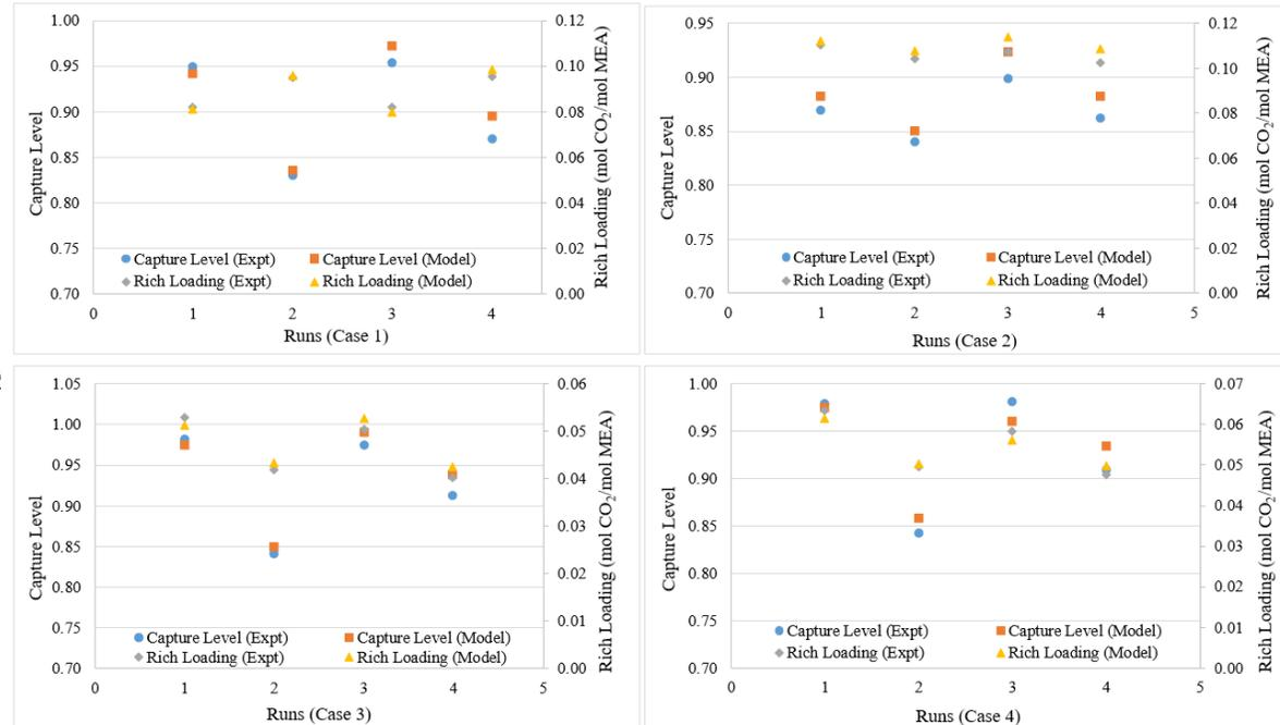
RPB absorber model validation for different cases from Jassim (2002)
