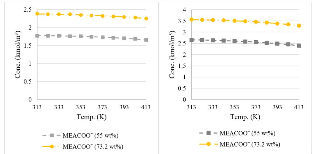
Liquid phase MEACOO<sup>-</sup> concentration at a loading of 0.2 (left) and 0.3 (right) for 55 and 73.2 wt% MEA solvent
