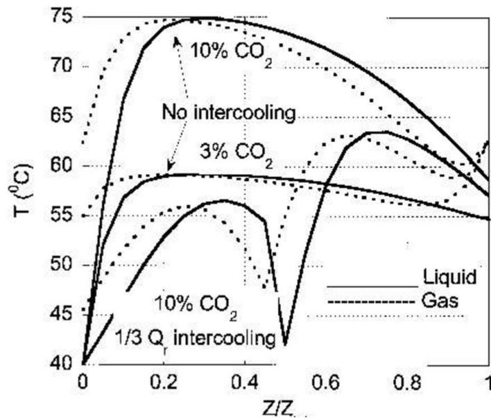
Absorber profile for conventional packed bed using 30 wt% MEA solvent (Freguia and Rochelle, 2003)
