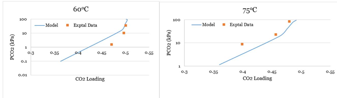
Model prediction for 74 wt% MEA solution with data from Aronu *et al.* (2011)
