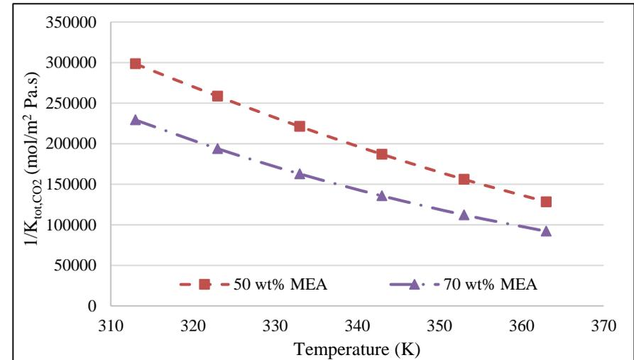
Mass transfer resistance for different temperature and concentrations
