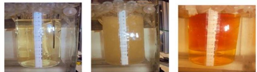
A 5M DEEA/2M MAPA solution: (a) before, (b) during, and (c) after CO<sub>2</sub> loading (Pinto et al., 2014)
