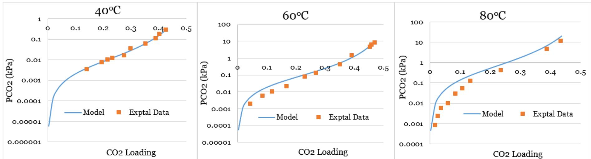
Model prediction for 45 wt% MEA solution with data from Aronu *et al.* (2011)
