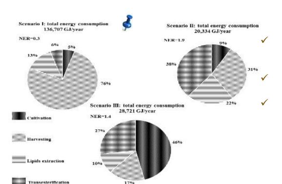
Microalgae require several process stages to be transformed into biodiesel Wastewater is a favourable option for cultivation If wastewater is used for cultivation, harvesting and lipid extraction+transesterification are the most energy intensive
