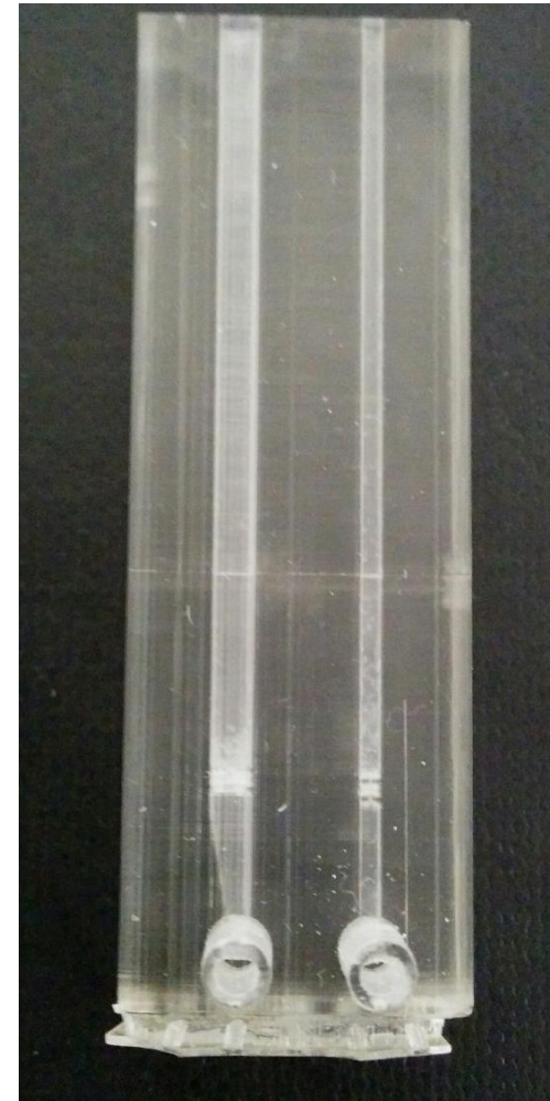
Final FB design with 4 layer of pillars; 2mm channel on left and 1mm channel on right
