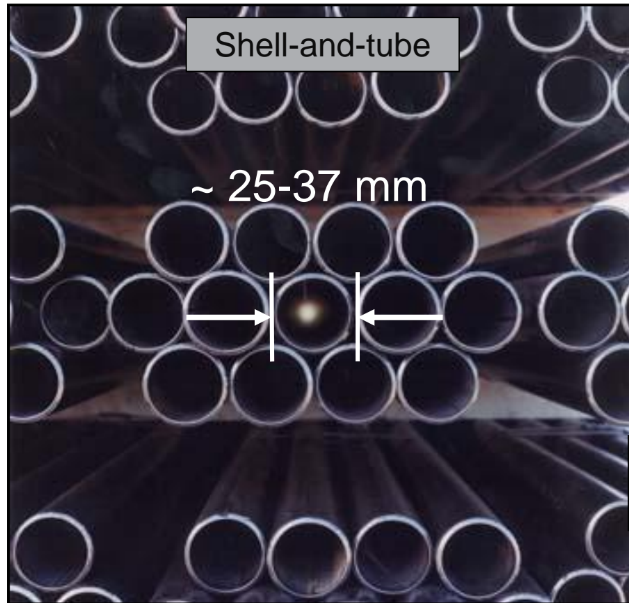
Conventional FT reactor Tube length 30+ feet (9+ meters)
