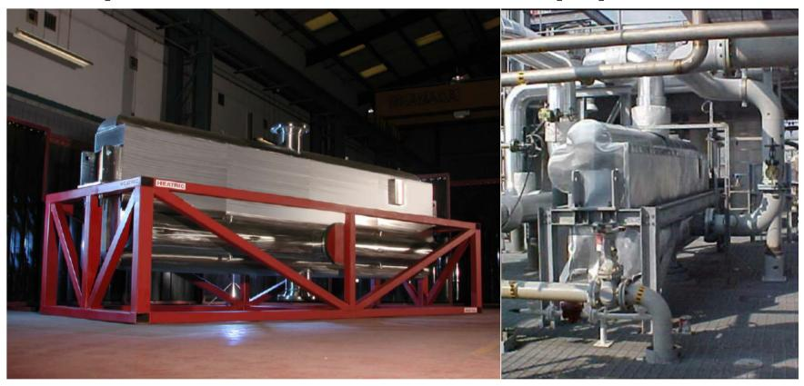
BASF Geismar Ethylene Oxyde Lean/Rich Exchanger
