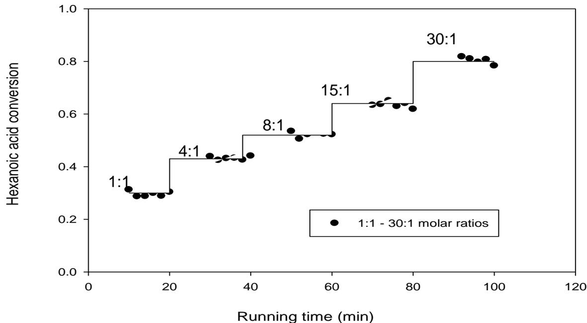
Continuous esterification of hexanoic acid with methanol in mesoscale oscillatory baffled reactor, using Amberlyst 70 catalyst at operating conditions of 60°C, 10mins residence time ( $\tau$ ), catalyst packing of 0.45g loading per millilitre of reactor volume, oscillatory conditions of 4.5Hz and 8mm ( $Re_o = 2400$ ), and reactants molar ratios ramped from 1:1 to 30:1 methanol to acid molar ratios
