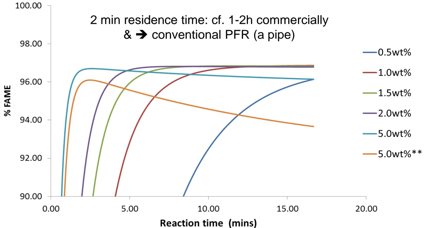
**Reaction time vs. FAME content as function of catalyst (KOH) concentration
