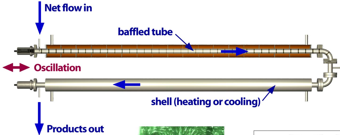
**Achieves plug flow by tanks in series rather than turbulence**
