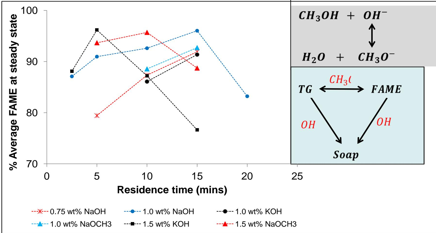
Effects of residence time on FAME (biodiesel) content at different catalysts concentrations for RSO transesterification at 6:1 methanol/RSO molar ratio,  $Re_0 = 160$ ,  $T = 60^\circ C$ .
