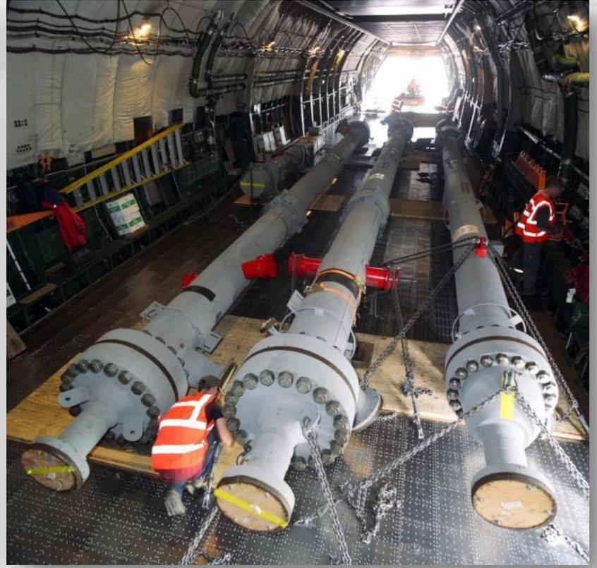
After 9 months of unsuccessful attempts to seal the heat exchanger flanges at the plant the original seal arrangement was scrapped. The Heat Exchangers were sent to Vector to be machined to accept techlok seals and flown direct to the plant in China. Where they were installed successfully and still remain in service.
