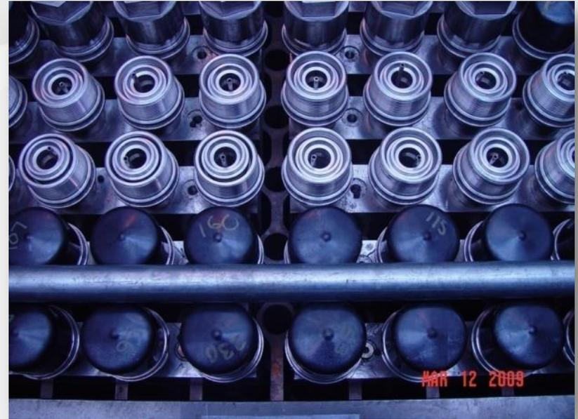
Specialist catalyst pipe closures custom developed for a high temperature prototype reformer chemical reactor that converts gas to liquid. The media was Hydrogen at 600°C. Banks of closures that require periodic opening and closing to install catalyst direct to the reactor. Low leakage to atmosphere was a key requirement. [service](#)
