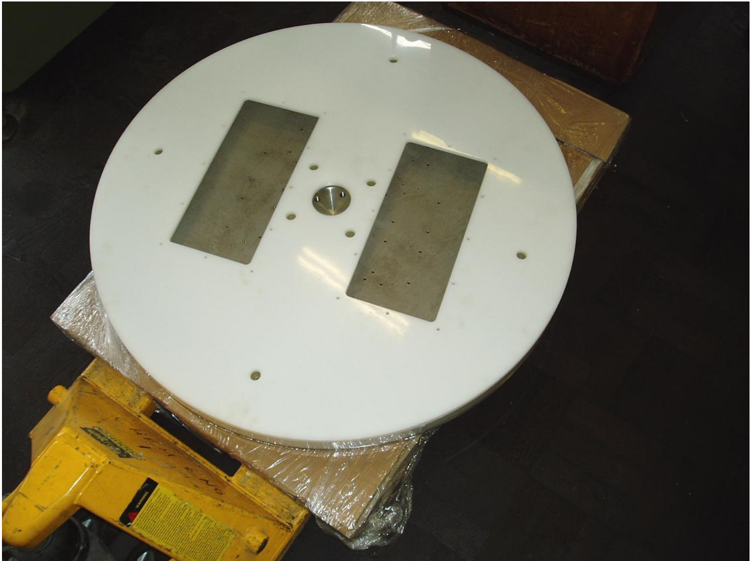
Support disc with instrument cover– data logger access panels remo
