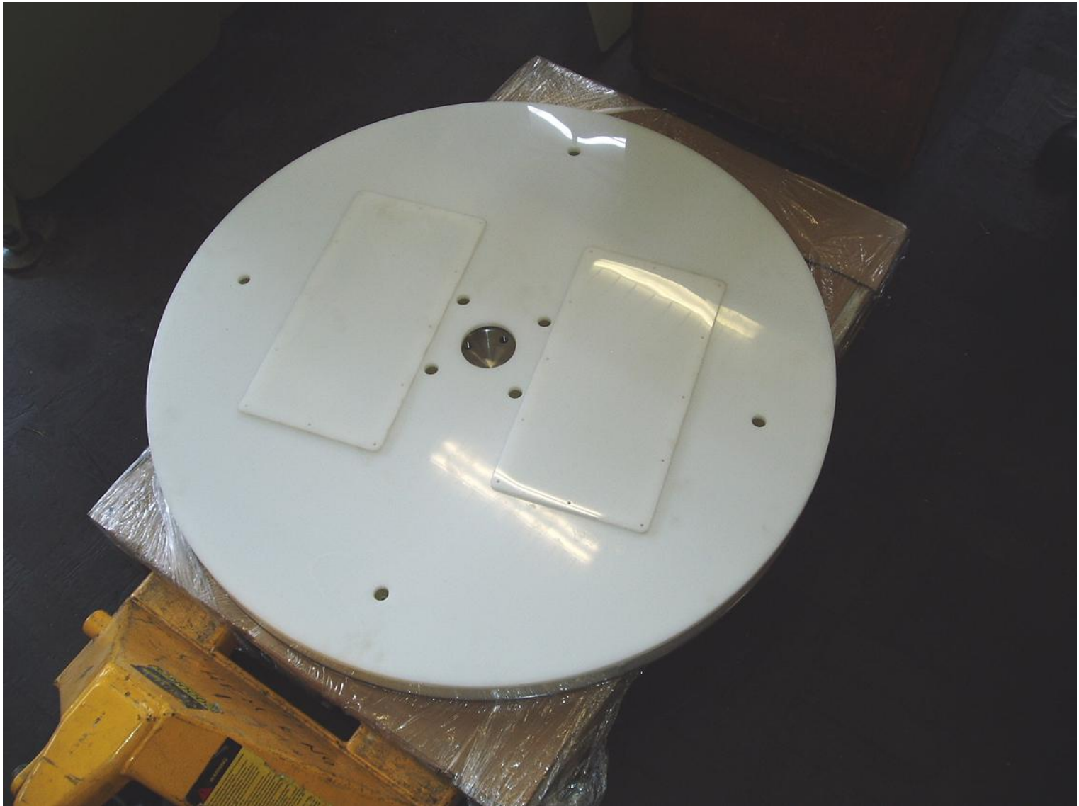
Support disc with instrument cover – data logger access panels in place
