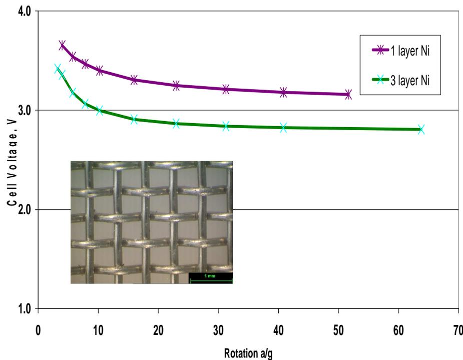
Current Density 13.5 kA/m<sup>2</sup>, 30% w/w KOH, Ambient Temperature, with 0.5
