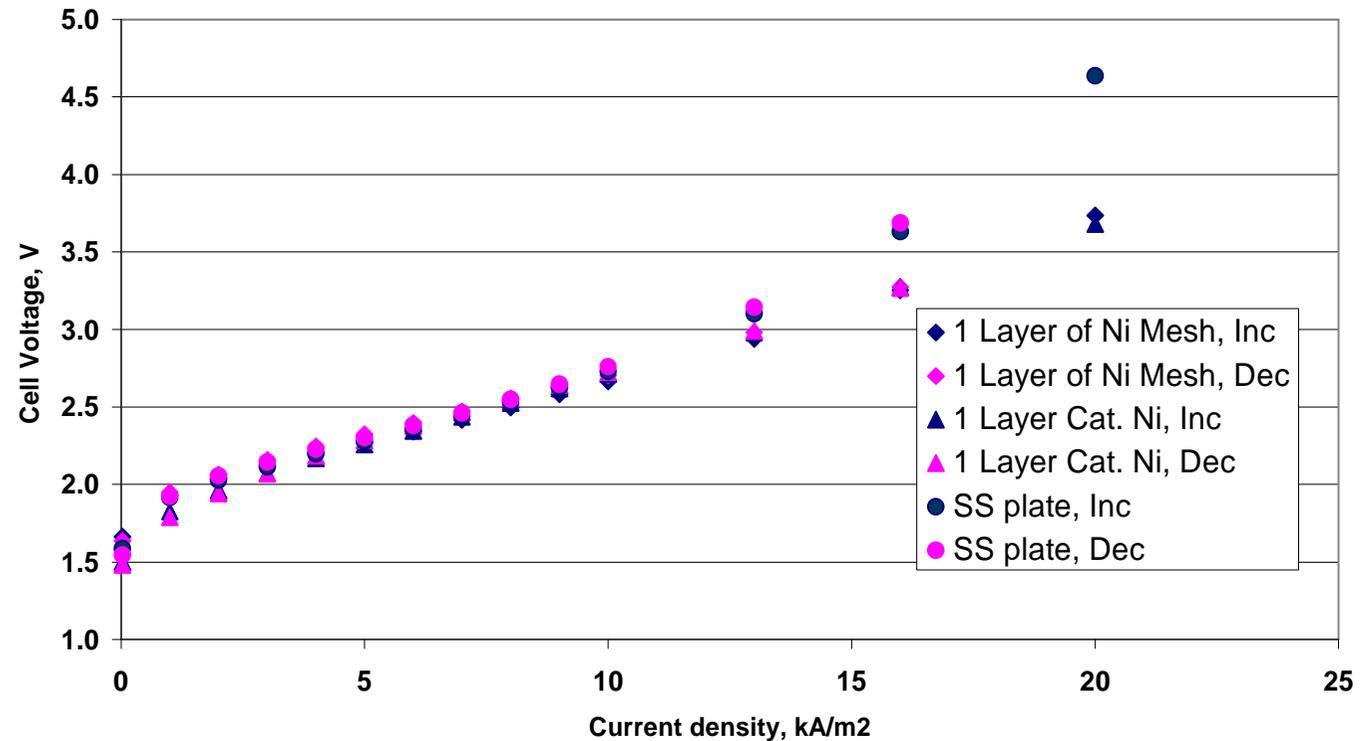
**Increase of actual area of electrodes helped to reduce the cell voltage, catalyst coating has little effect**
