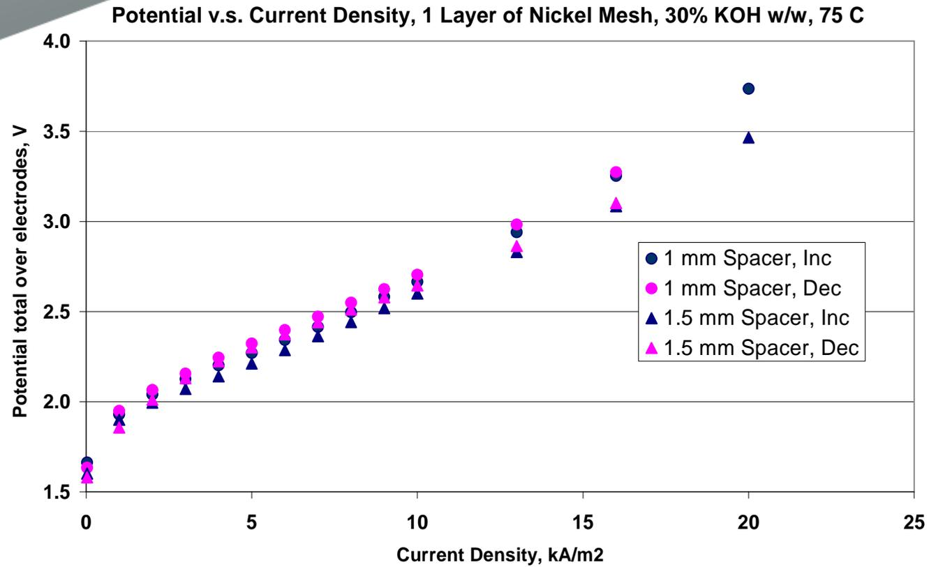
Extra space for gas removal reduces cell voltage
