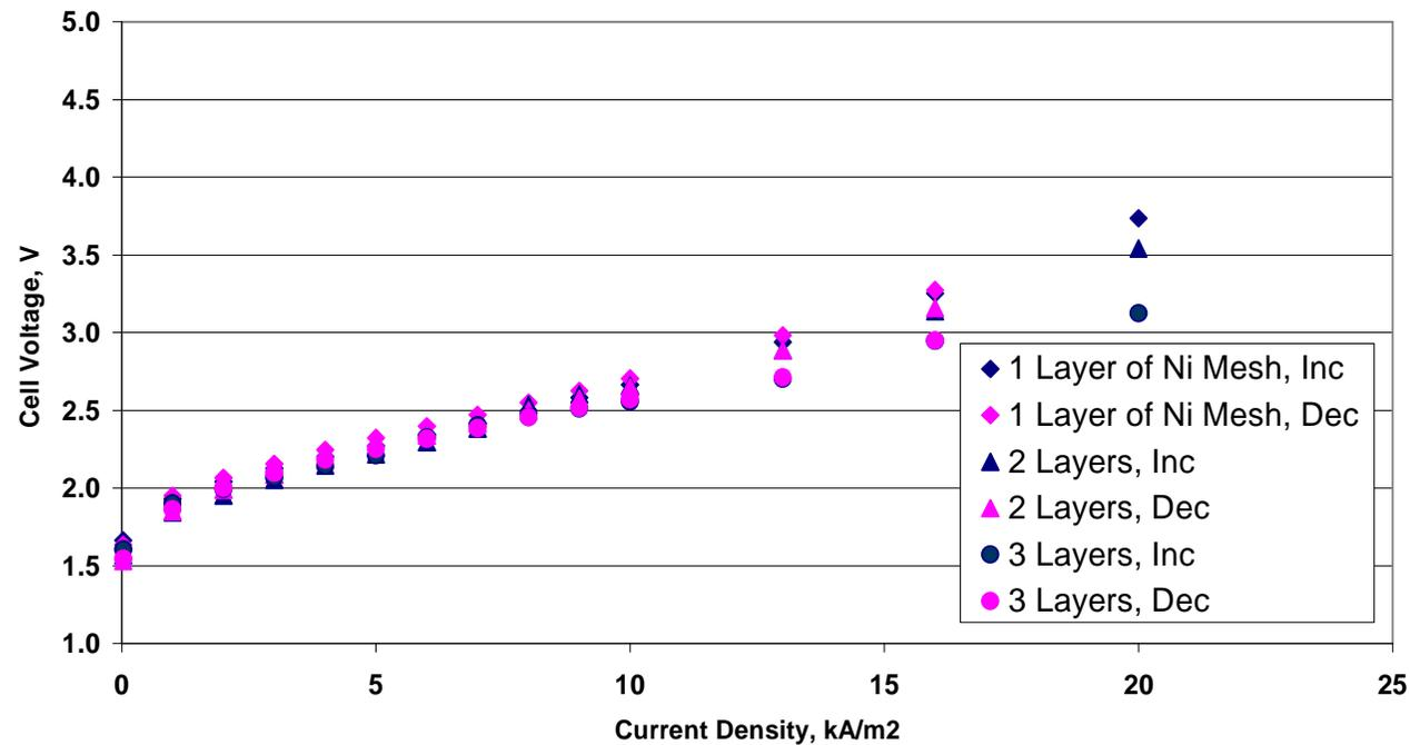
Extra mesh layers reduces cell voltage especially at high current density
