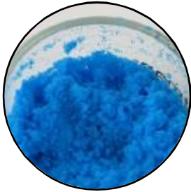
PVA, 50-200 \mu\text{m} , 1.4 \text{g}/\text{cm}^3
